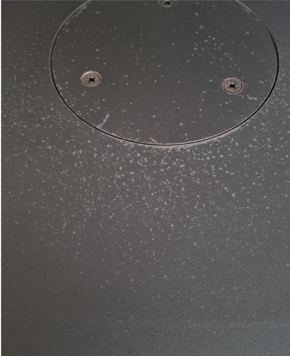
All stoves on the market are either made from mild steel or cast iron. The mild steel models like this are shot blasted and then painted with high temperature black paint. This will protect the stove but if the stove remains damp or wet for a long time the oxidization process ( surface rusting ) will begin.
