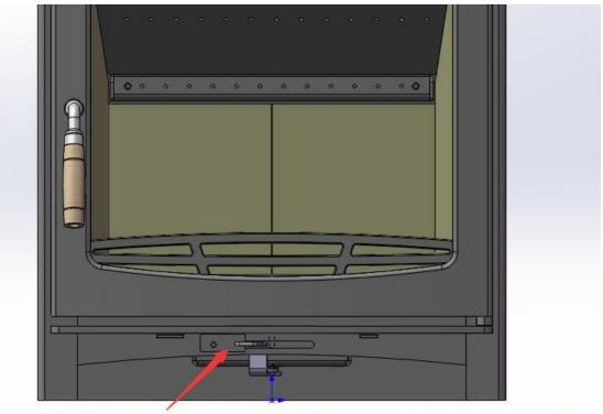
This is 18mm stop plate, we could take off or reverse placing when we need standard version.
